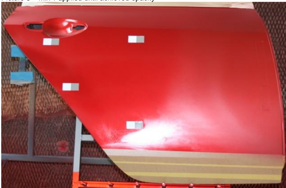
Picture 3 – Mix 1 applied until achieved opacity
