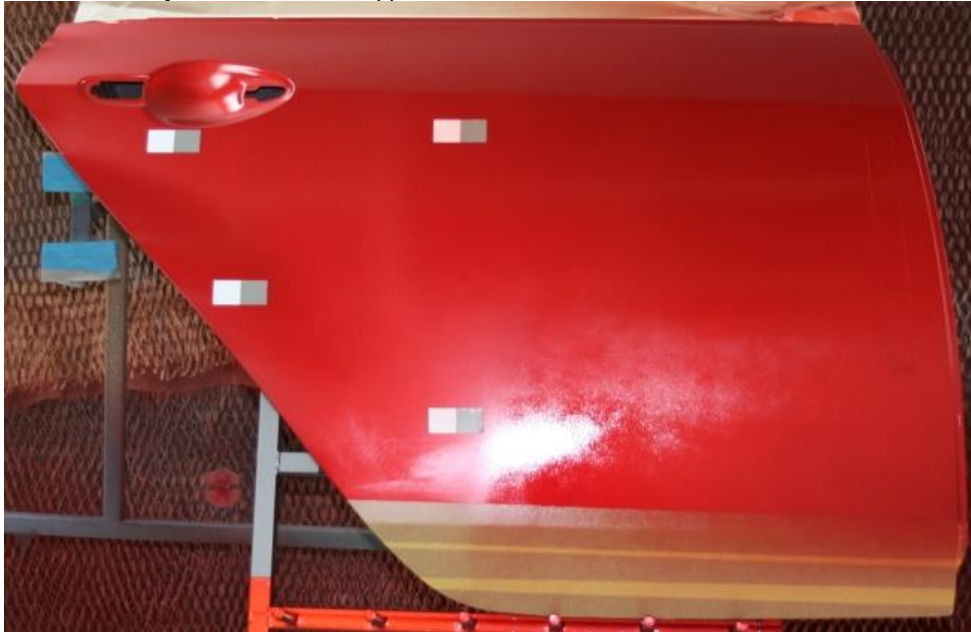
Picture 4 – 2 layers of Effect coat applied
