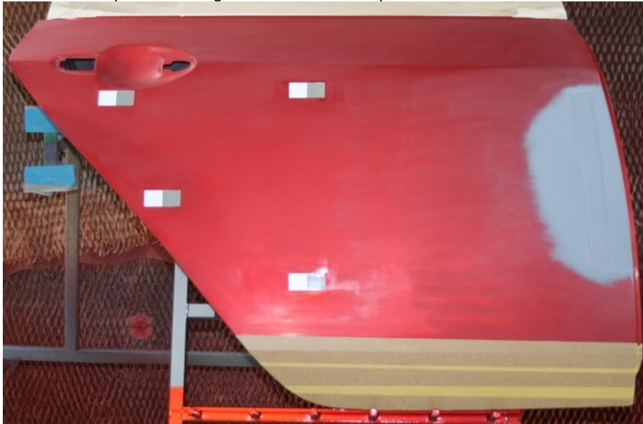
Picture 1 – Prepared and degreased area under repair
