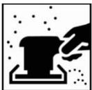
Remove existing coating and sand down to the bare substrate using P120 - P220 grit as the final step.
