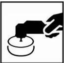
Thoroughly polish the blending area with an abrasive polishing compound, preferably in combination with a polishing machine.
