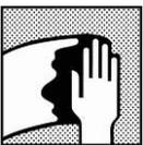
Remove any surface contamination with an appropriate surface cleaner prior to topcoat/clearcoat application.
