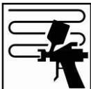
Apply 1-3 thin coats on the blending area, extending forward into the polished area.
