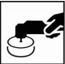
Polish the blended area by hand or machine using a fine polishing compound.
