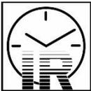
Allow 15 minutes flash off prior to infra red curing.
