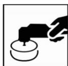
Dust and minor imperfections can be polished out after the stated air-dry times have been reached, or after a full bake at 60°C object temperature, followed by a cool down of the object to ambient temperature. Carefully sand out dust particles and restore the surface according polishing recommendations. Ready to polish approximately 30 minutes after cool-down to ambient temperature.
