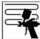
Apply a medium closed coat, allowing for a 5-10 minutes flash-off time at 25°C.
