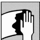
Surface cleaning; remove any surface contamination prior to the application of Spotprimer DTM using Sikkens M700 or M600 surface cleaner. Where bodyfiller is exposed, avoid contact with water (e.g. waterborne degreaser).
