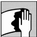
Surface cleaning; remove any surface contamination prior to sanding using Sikkens M700 or M600 surface cleaner.
