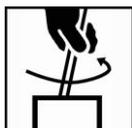
The Autowave MM colors must be stirred thoroughly directly after mixing the formula.
