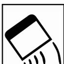
Apply Polyfiber to bare substrate at a 60° angle.
