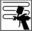
Apply a medium closed coat, allow for 3-10 minutes flash-off and apply a full coat.
