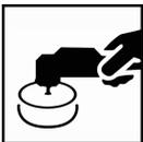
Dust and minor imperfections can be polished out after the stated air-dry times have been reached or after a full bake at 60°C object temperature, followed by a cool down of the object to ambient temperature.
