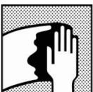
Surface cleaning; remove any surface contamination prior to the application of the topcoat using an appropriate surface cleaner.
