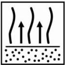
Allow for a minimum flash-off time of 15 minutes at 20°C prior to topcoat application.
