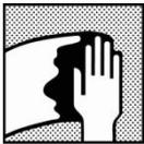
Surface cleaning; remove any surface contamination prior to Colorbuild application using appropriate surface cleaner. *Where bodyfiller is exposed, avoid contact with water (e.g. waterborne degreaser).*
