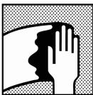
Remove contamination using an appropriate cleaner.
