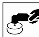
Dust and minor imperfections can be polished out after the stated air-dry times have been reached, or after a full bake at 60°C object temperature, followed by a cool down of the object to ambient temperature. Carefully sand out dust particles and restore the surface according polishing recommendations. Ready to polish approximately 1 hour after cool down to ambient temperature.
