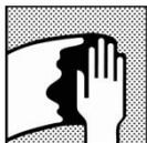
Surface cleaning; remove any surface contamination prior to Colorbuild application using Sikkens M700 or M600 surface cleaner.
