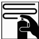
Hold aerosol approximately 12 – 18 cm from the panel and apply 2 – 3 even coats. *Autosurfacers UV is transparent to allow proper curing of the filler. **Do not spray until hiding. Too much layer thickness may cause adhesion failures due to insufficient through cure.***
