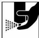
After application, invert aerosol and depress the nozzle for 2-3 seconds. *This allows the propellant to clean the nozzle sufficiently for further use*
