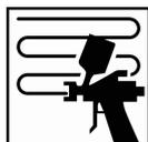
Apply two single coats, allowing for a 0-3 minutes flash-off time at 20°C between coats
