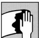
Surface cleaning; remove any surface contamination prior to the application of the topcoat using an appropriate surface cleaner.
