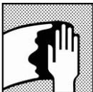
Surface cleaning; remove any surface contamination prior to Autosurfacer UV application using appropriate surface cleaner. *Where bodyfiller is exposed, avoid contact with water (e.g. waterborne degreaser).*
