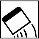
Apply the Polyfiber to a bare substrate at a 60° angle.
