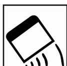
Apply Polysoft Plastic to the bare plastic at a 60° angle.
