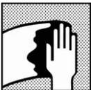
Surface cleaning, remove any surface contamination prior to the application of Rally Black using an appropriate surface cleaner.
