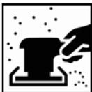
Remove existing coating and sand down to the bare substrate using P180 - P220 grit as the final step.
