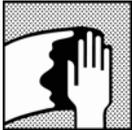
Remove any surface contamination prior to sanding application using appropriate surface cleaner.
