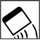
Apply the polyester bodyfiller to the bare plastic substrate by placing the spreader at a 60° angle. Avoid thick edges of bodyfiller around the perimeter of the repair by tapering away toward the original finish.
