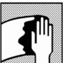
Remove any surface contamination prior to filler / surfacer application using appropriate surface cleaner.
