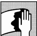
Surface cleaning, remove any surface contamination prior to putty/bodyfiller application using appropriate surface cleaner.
