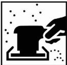
Remove existing coating and sand down to the bare substrate using P180 - P280 grit as the final step.
