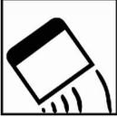
Apply the polyester bodyfiller to the bare substrate by placing the spreader at a 60° angle. Avoid thick edges of bodyfiller around the perimeter of the repair by tapering away toward the original finish.
