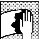
Remove any surface contamination prior to primer, filler or surfacer application using appropriate surface cleaner. *Where bodyfiller is exposed, avoid contact with water (e.g. waterborne degreaser).*
