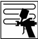
**Sanding;** Apply one coat over the total sanded area. Next apply the 2<sup>nd</sup> and 3<sup>rd</sup> coat within each preceding coat. Where a full panel application is required apply 2-3 coats over the total panel dependent on the required film build.
