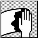
Surface cleaning; remove any surface contamination prior to Colorbuild application using Sikkens M700 or M600 surface cleaner. *Where bodyfiller is exposed, avoid contact with water (e.g. waterborne degreaser).*
