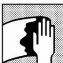
Surface cleaning; remove any surface contamination prior to the application of the topcoat using Sikkens M700 or M600 surface cleaner for. In case of Autowave application also clean with M850 Solfree or M200.
