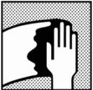
Surface cleaning; remove any surface contamination prior to Colorbuild application using Sikkens M700 or M600 surface cleaner. Where bodyfiller is exposed, avoid contact with water (e.g.M850 Solfree or M200).
