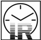
Allow 5 minutes flash-off prior to infra red curing
