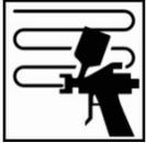
Allow each coat to flash-off naturally until the surface is completely matt; this also supports to achieve higher film build. Do not force-dry by air support. Flash-off between the coats is dependent on ambient temperature, applied layer thickness and airflow. For maximum build use large fluid tip and lower the application pressure.
