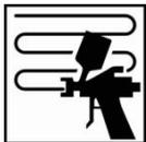
Apply 1 even coat over untreated plastic substrates.
