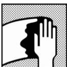
Surface cleaning; remove surface contamination using M700 or M850 or M200.
