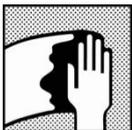
Pre-clean the surface with warm water and detergent and rinse sufficiently with clean water.
