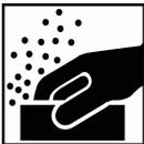
Abrade the surface by using minimum P400 dry sanding grit as the final step.
