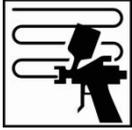
Apply a medium closed coat, allowing for a 3-5 minutes flash-off time at 20°C.
