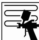
Apply one coat over the total sanded area. Next apply the 2<sup>nd</sup> coat within the previous coat.
