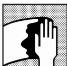
Surface cleaning, remove any surface contamination prior to the application of Autosurfacer Rapid using appropriate surface cleaner. *Where bodyfiller is exposed, avoid contact with water (e.g. waterborne degreaser).*
