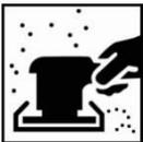
Remove existing coating and sand down to the bare substrate using P180 - P220 grit as the final step. For detailed surface preparation see TDS S8.06.02
