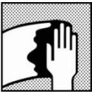
Remove any surface contamination prior to sanding application using appropriate surface cleaner. Pre-clean the surface with warm water and detergent, rinse sufficiently with clean water.
