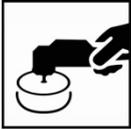
Dust and minor imperfections can be polished out after the stated air-dry times have been reached, or after a full bake at 60°C object temperature, followed by a cool down of the object to ambient temperature. Carefully sand out dust particles and restore the surface according polishing recommendations. Ready to polish approximately 1 hour after cool down to ambient temperature.
