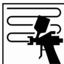
Apply a medium closed coat, allowing for a 3-5 minutes flash-off time.
