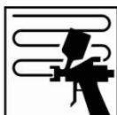
Apply a medium closed coat, allowing for a 5-10 minutes flash-off time at 20°C.
