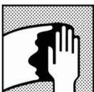
Surface cleaning, remove any surface contamination prior to the application of a primer surfacer using Sikkens M700 or M600 surface cleaner. Where bodyfiller is exposed, avoid contact with water (e.g. waterborne degreaser).
