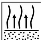
Allow for a 4-8 minutes flash off time between coats at 20°C.
