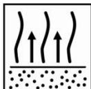
Allow for a minimum of 15 minutes flash off time at 20°C before recoating.
